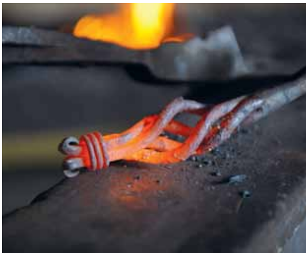
Iron is reheated to reduce its brittleness
