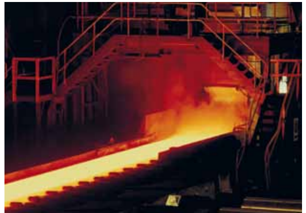
A hot strip mill run-out table
