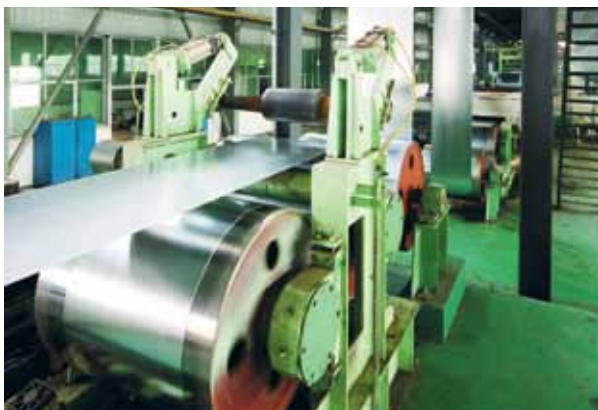
A steel coil galvanising production line
