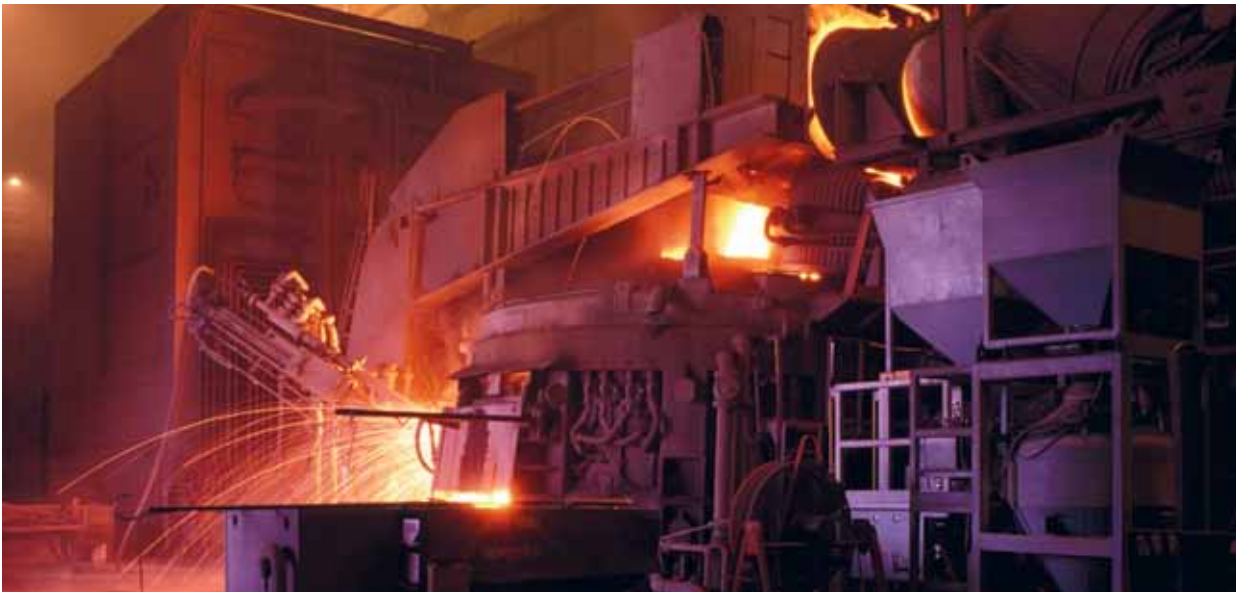
An Electric Arc Furnace (EAF)
